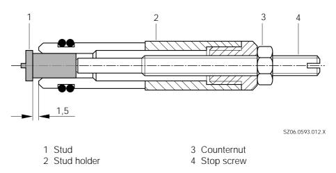
If other stud diameters are used, different stud holders matching the stud diameters are required.
